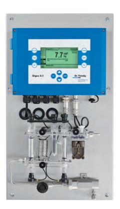
Measuring hydrazine concentrations in high-purity water
