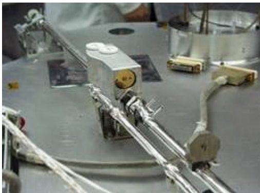
Figure 4 TDL System mounted on the Mars Polar Lander
