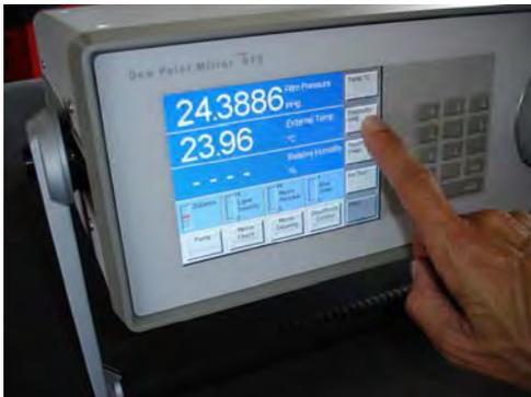
3. Change other units (such as pressure, flow rate, etc.) with the same method.
