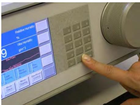
1. Press and hold the *enter* key on the numeric keypad for 3 or 4 seconds. If you've done it correctly, you'll hear two loud short beeps. If not, release the key and try again.
