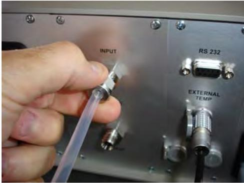
The input and output connectors are clearly labeled on the Sample Gas section of the back panel. Depending on the specific model and ordered options, the stainless steel gas input and output connections may be 6 mm Swagelok, ¼ inch Swagelok, or ¼ inch Cajon VCR.
