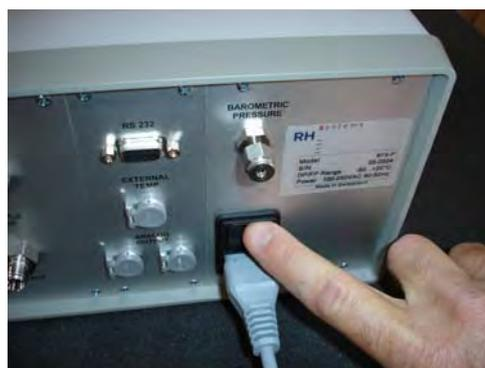
The display should become visible within a few seconds. If nothing seems to happen, check the power source. There may also be some fuses located next to the power switch. You can remove and replace them with known good ones. Suspect fuses can be tested for continuity with an ohmmeter.
