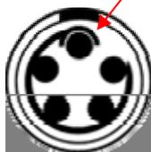
If you wish to connect your own thermometers, the 973 requires a 5 pin connector, LEMO ([www.lemo.ch](http://www.lemo.ch)) part number FGG 1B 305 CLAD 42.
