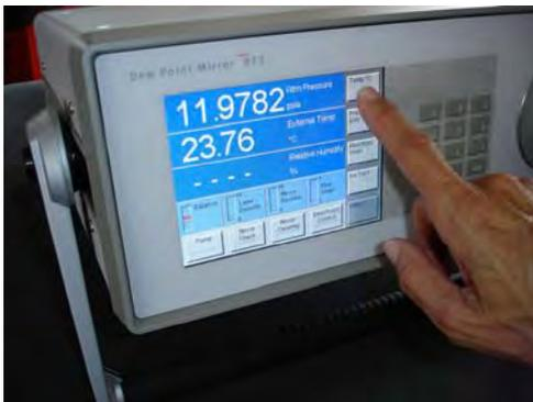
2. To change temperature units, press the key labeled 'Temp'. Notice that the corresponding units change each time the key is pressed. Also notice that any data line that is currently indicating temperature data also changes to reflect the newly selected units.
