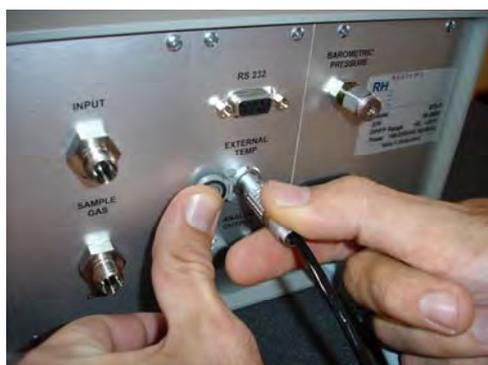
The 973 is equipped with an external temperature sensor. This sensor, along with the dew point and pressure measurement, allows the 973 to accurately determine and display relative humidity. The external temperature probe connection is made at the back panel.
