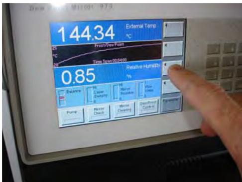
2. Press the arrow key corresponding to the data line you wish to change. Notice that each time you press the arrow key, the parameter of the data line changes. The parameter selection is circular, meaning that once you reach beyond the last available parameter the first one is again displayed and the cycle starts over.
