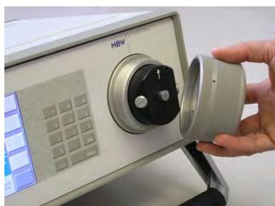
The measuring head is located on the right side of the 973 front panel. To gain access to the mirror and opto-electronic components, you must first remove the cover screw by twisting it counterclockwise. It requires approximately three full turns to completely unscrew, allowing you to remove it.
