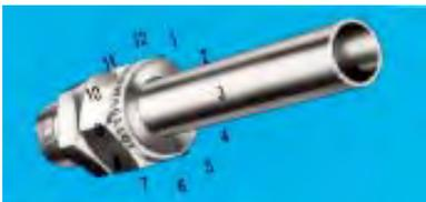
Before tightening the SWAGELOK® nut, scribe the nut at the 6 o'clock position.
