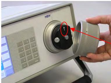
1. Install the optical assembly, taking note of guide pin.
