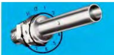
Hold the fitting body steady with a backup wrench and tighten the nut 1-1/4 turns. ① Watch the scribe mark, make one complete revolution and continue to the 9 o'clock position. By scribing the nut at the 6 o'clock position as it appears to you, there will be no doubt as to the starting position. When the nut is tightened 1-1/4 turns to the 9 o'clock position, you can easily see that the fitting has been properly tightened.
