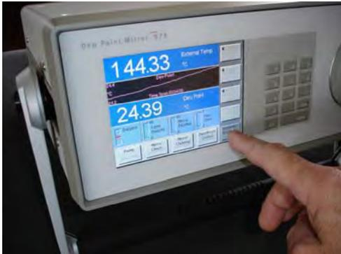
1. Use the lower right menu key to select the **Numeric/Graphic** menu. 'Numeric/Graphic' appears on the key, and the keys above contain left pointing arrows. Notice that each key corresponds to the data line it points toward.
