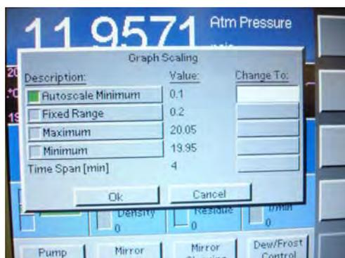
Each graph can have its own scaling (or y-axis) values. There are three distinctly different scaling modes to choose from:
