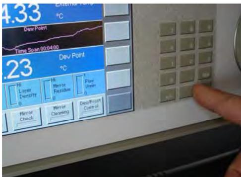
4. If you like, you may clear the menu keys when finished by cycling through all the menus using the lower right key on the touch screen, or by pressing the *enter* key once. Note that this is not required and nothing is wrong with leaving the Parameter menu (or any other menu) on the screen.
