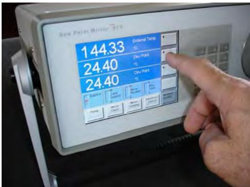
3. Select numeric or graph mode on any of the other data lines with the same method. [Notice that if a line is currently displaying the Status Bar, no arrow appears on the adjacent menu key. The Status Bar is not changeable in the Numeric/Graphic menu.]
