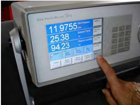
1. Use the lower right menu key to select the **Units** menu. 'Units' appears on the key, and the keys above contain current units indications such as 'Temp °C'. Notice that each of the keys contain different types of units. In this case, the keys do not correspond to the adjacent data lines, but rather to different units types.
