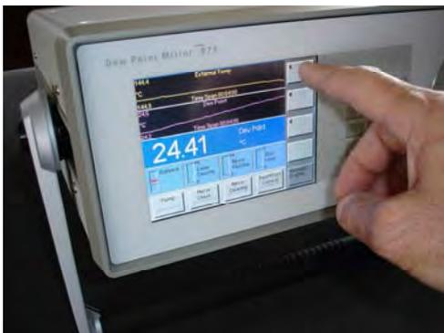
2. Press the arrow key corresponding to the data line you wish to change. Notice that the data line toggles between numeric or graph mode each time you press the key.
