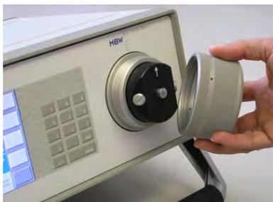
The heart of the 973 Dew Point Mirror instrument is the measuring head assembly. It is designed to be highly sensitive and accurate, yet rugged and easily accessible for periodic mirror cleaning. Although not required prior to initial operation, you may wish to familiarize yourself with the location and accessibility of the mirror and the other optical components within this assembly.
