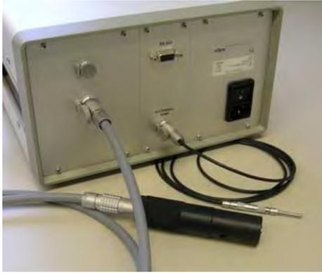
Use the optional 5 pin temperature probe cable to connect the external temperature probe directly to the 473 back panel.
