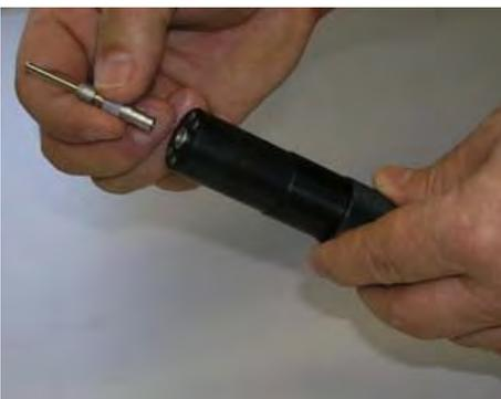
The External Temperature probe is usually directly connected to the 473 measuring head.
