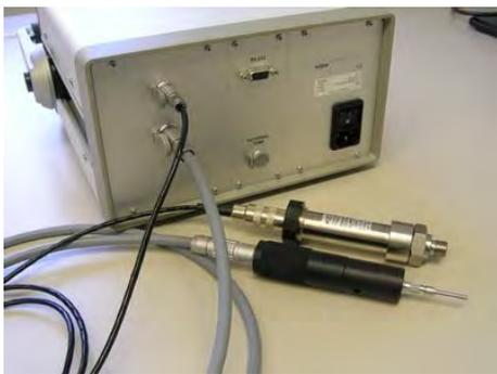
Use the 5 pin cable to connect the pressure sensor to the 473 back panel.
