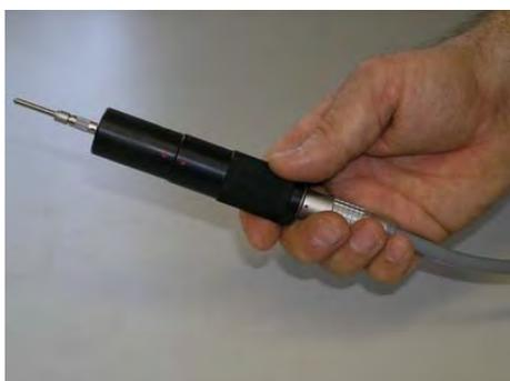
To gain access to the mirror and opto-electronic components, you must remove the optical assembly from the measuring head. The two red dots indicate where the measuring head and optical assembly will separate.
