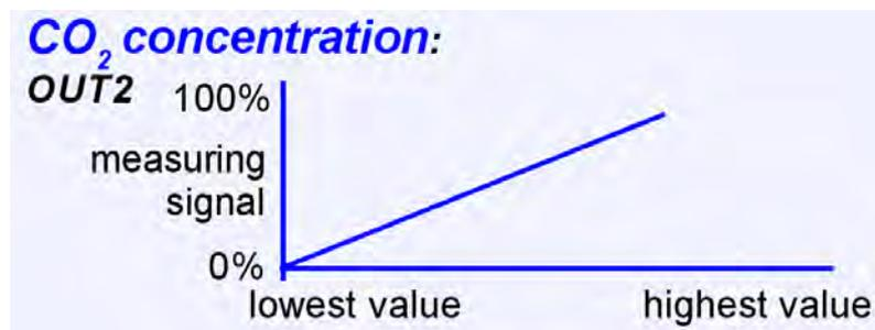
Figure 2. The measuring signal of carbon dioxide.
