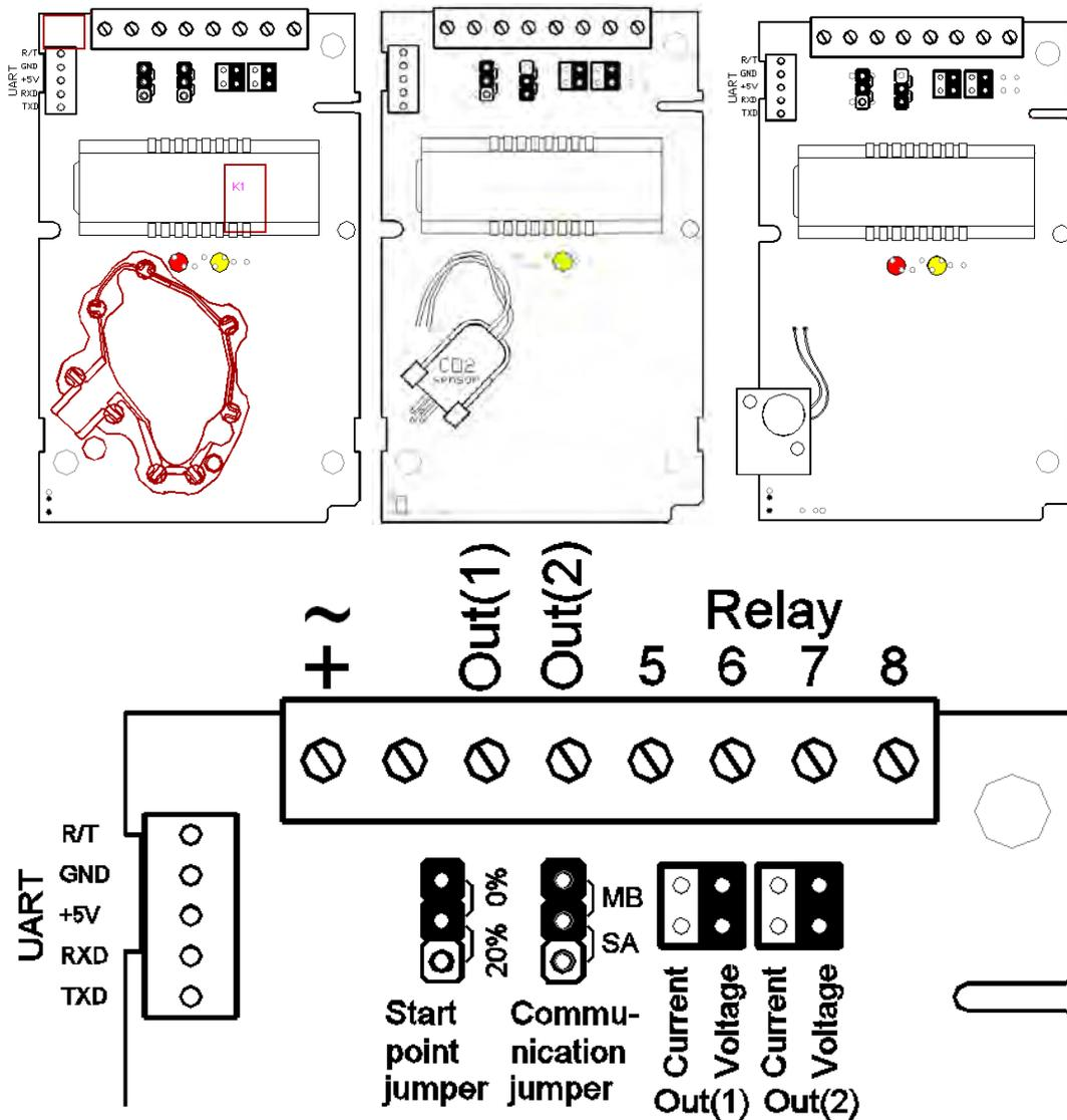
Figure 6. The CF8-W-Disp-GH printed circuit board with CO<sub>2</sub> sensors for measuring ranges 0-3000ppm, 0-10% och 0-25%. The terminal area enlarged at right. The darker positions are default settings.
