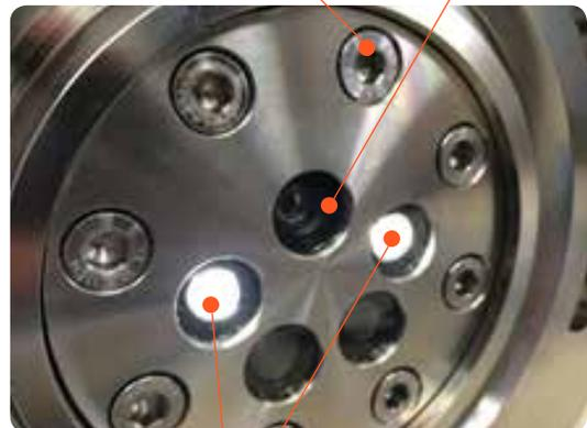
Two LED ports for illumination, two spare ports for future upgrades
