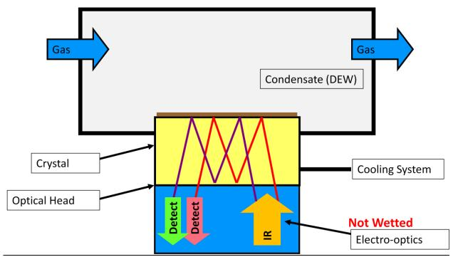
ZEGAZ Instruments CEIRSTM Principle of Operations
