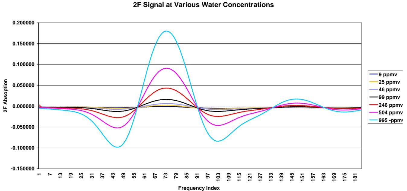
**FIGURE 2. 2F ABSORPTION SIGNALS AT VARIOUS MOISTURE CONCENTRATIONS**
